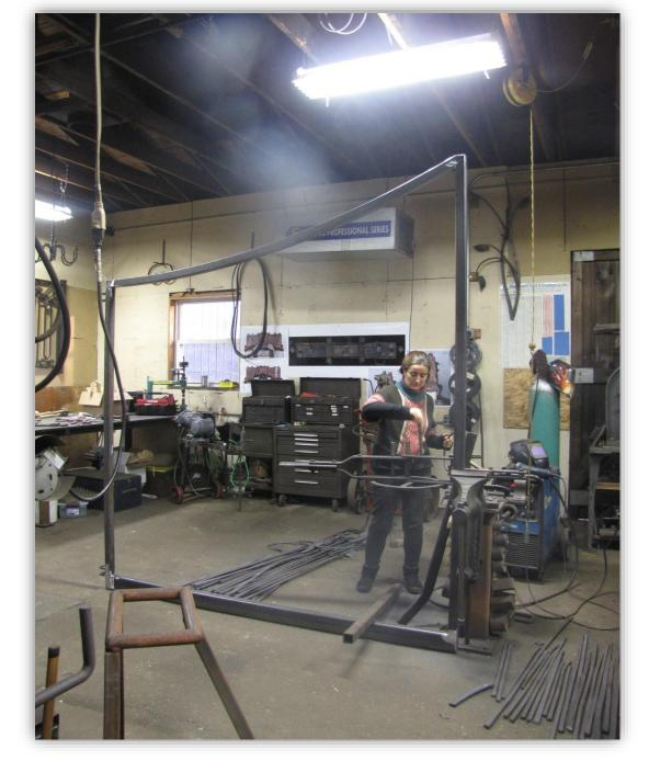
The empty gate frame was fabricated and set up in the middle of the shop. The leaves and stems that were to be fitted into the frame were placed on the floor for easy access. This allowed the fabricator to work efficiently between the anvil, vice, drawing and frame.
