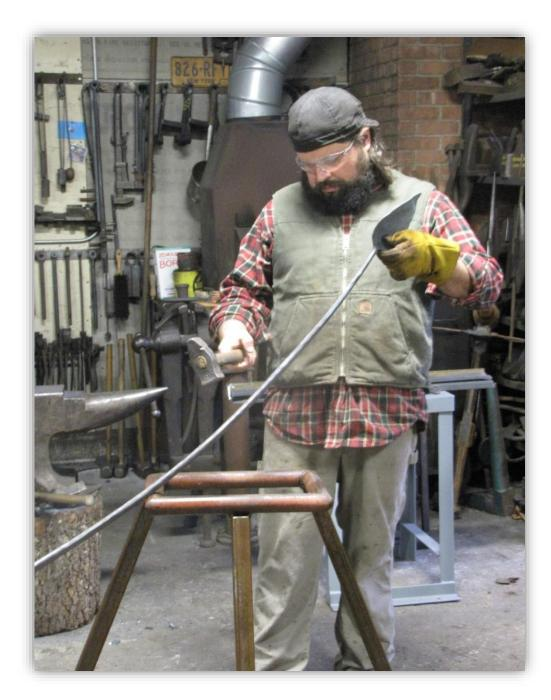
This was most easily accomplished by using a traditional tool called a French bending anvil. The smith had a much more subtle control than using hydraulics or mechanical means of bending.
