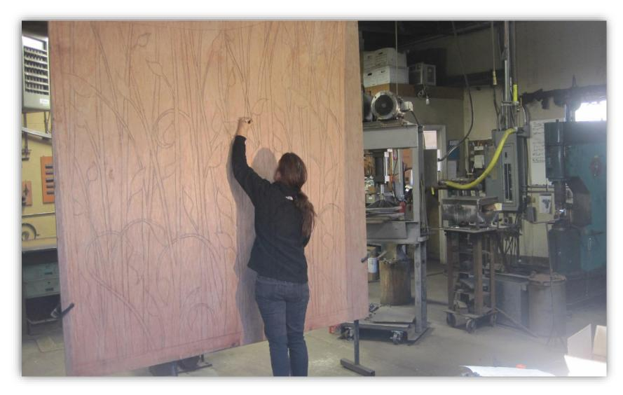
The owner and lead designer, Rachel Miller had transferred the design drawing to several large sheets of plywood in order to create a full size drawing of the driveway gates. This allowed our blacksmiths/fabricators to efficiently translate the design into a set of working driveway gates.
