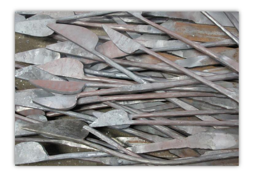
Here you can see that our blacksmith has forged a large portion of the 150+ leaves and stems needed to fill the 2 gate panels. Each stem was bent to its own individual curve as laid out in the design.
