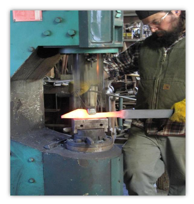
Our master smith Timothy Miller had to construct special tooling to efficiently forge such a large quantity of leaves and stems needed for the custom gate. Here, he is setting the shoulder that forms the bottom part of the leaf using a large, self-contained power forging hammer. Methods like this have their origins in heavy industry. Spirit Ironworks have turned these methods to the service of art.
